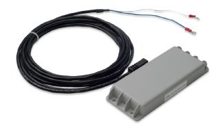
This unique device senses when it is connected to external power and can be programmed to send its location more frequently.
